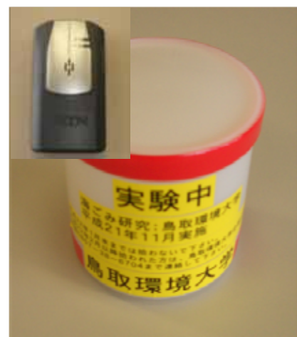
Fig. 2 The plastic bottle and the transmitter used
