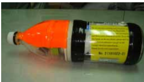
Fig. 4 GPS transmitter-containing PET bottle
